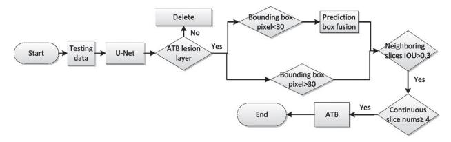
Fig. 4. AI detection software - diagnostic flowchart.
