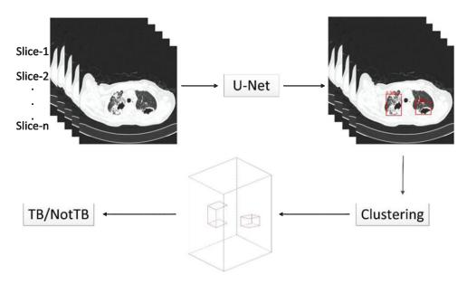
Fig. 2. Main framework of AI detection software.
