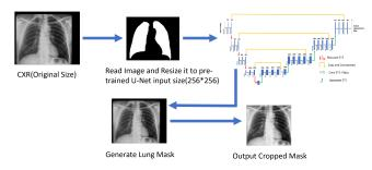
Fig. 1: Preprocessing pipeline for CXRs
