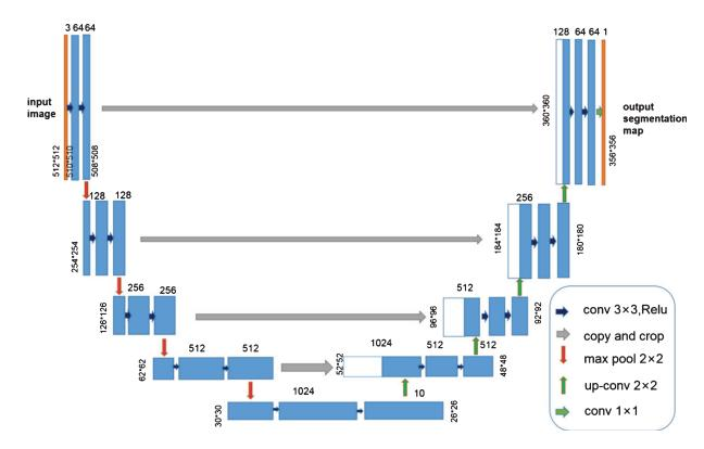
Fig. 3. Architecture of our adapted U-Net network.
